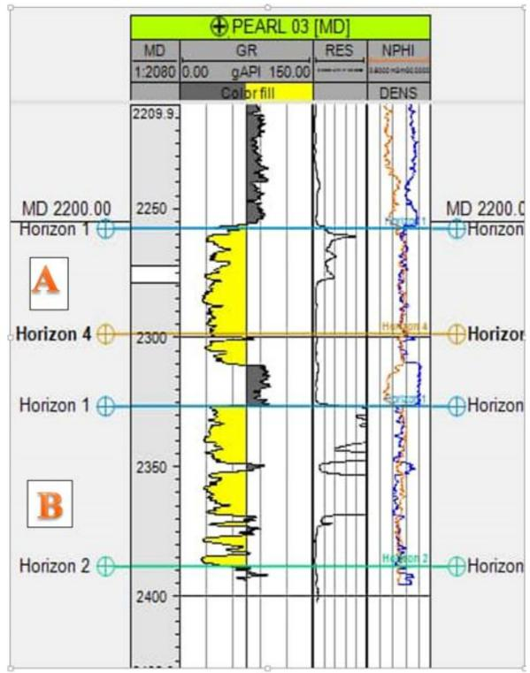
Figure 5. Log Display of Reservoir A and B in well (Pearl) 03, using Petrel 2015 software.
