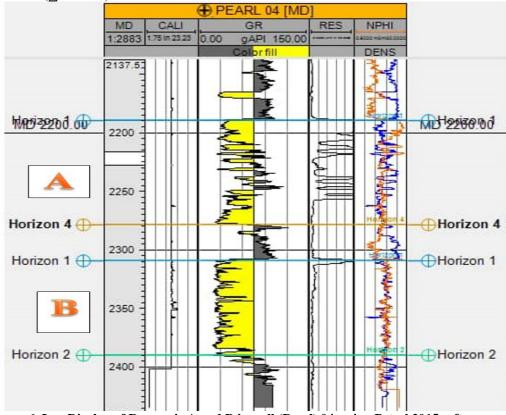
Figure 6. Log Display of Reservoir A and B in well (Pearl) 04, using Petrel 2015 software.
